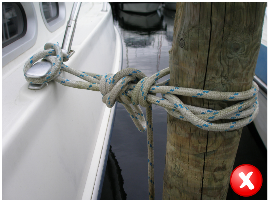
short mooring lines don't allow for water level changes
